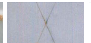
Samsung's rust-free cabinet material after 1000 hours
